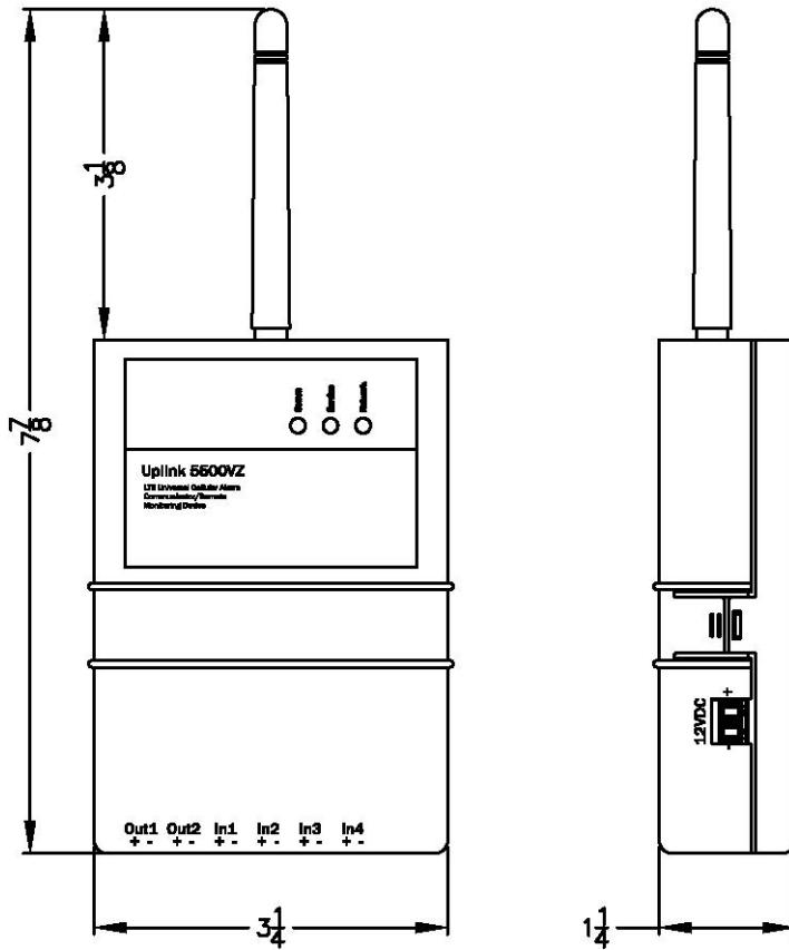
\* Note: Support for up to 4 input circuits and 2 output circuits. Consult the factory for available configurations. Standard configuration assumes high-water-alarm only.
