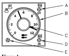
**Figure 1:** Adjustment screws/dials
