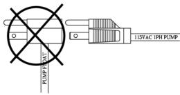
Figure 3: Not compatible with piggyback float plugs (See 10A650 for alternative)
