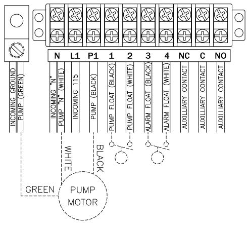
\*\*PUMP AND PUMP FLOAT TERMINALS NOT FOR USE WITH PIGGYBACK FLOATS, PLUG MUST BE REMOVED OR INSTALLED TO EXTERNAL OUTLET. PUMPS WITH BUILT—IN FLOATS REQUIRE JUMPER WIRE BETWEEN TERMINAL BLOCKS #1 AND #2
