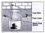
Figure 2: General tank setup
